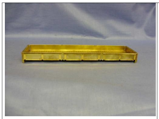
Fold over the top of the body sides to form a lip and bend the bottom of the body sides to 90 degrees. Now fit the ends and sides to the wagon bed . To gauge the correct place to solder the sides to the wagon bed, test fit the solebars by offering these up to the underside of the wagon bed and ensure that the bottom side of these are level with the bottom of the ends. See the picture two pages on if in any doubt.
