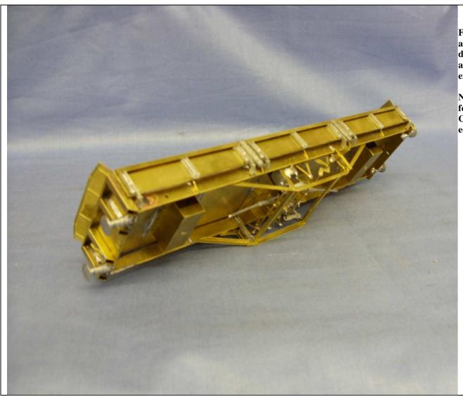
Fit the buffers and lamp brackets to each end and also the brass end ramps. Fit the later by folding down the three flaps and solder these into the slots at the top of the wagon ends. Note that the outer ends of these should be bent upwards first.
