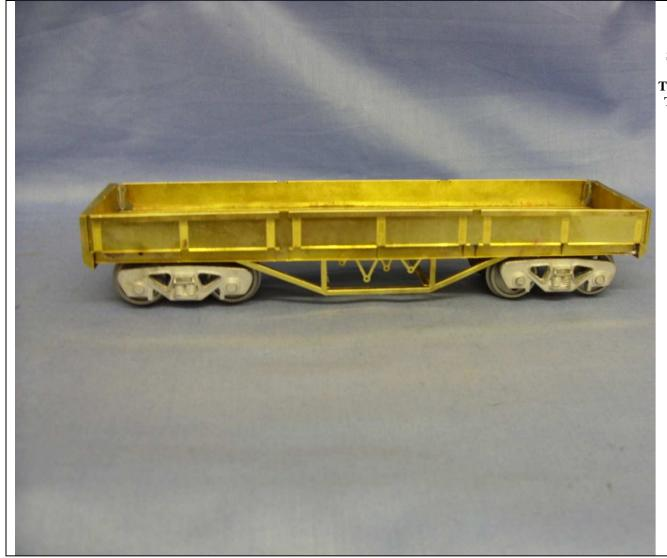
Solder the truss rod assembly to the rear of the solebars and wagon bed in the position shown.
