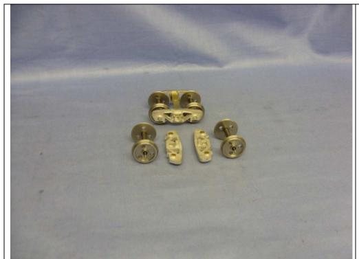
Make both bogies remembering to fit the top hat bearing. The cross brace is an etch brass part. This can be seen on the completed bogie.
